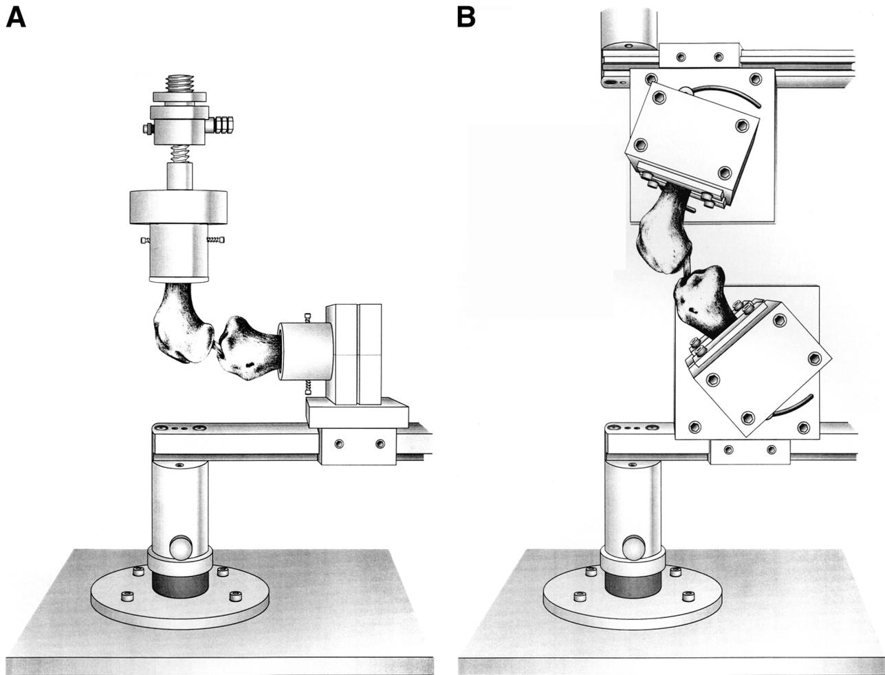
**FIGURE 2.** (A) The knee mounted in  $90^\circ$  to the materials testing machine for AP drawer testing. (B) The femur-ACL-tibia construct for failure testing with a flexion angle of  $60^\circ$  and the graft aligned parallel to the axis of the applied load. The adjusting device allows free rotation under different flexion angles.
