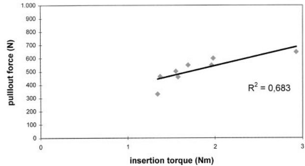
**FIGURE 6.** Correlation between pullout force and insertion torque for the biodegradable direct tendon fixation.
